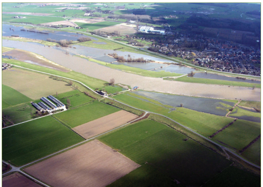
Figure 5. River IJssel is part of the 'Room for the river' programme, which is designed to accommodate an extra 22 600 m 3 /s discharge from the Rhine and Meuse
